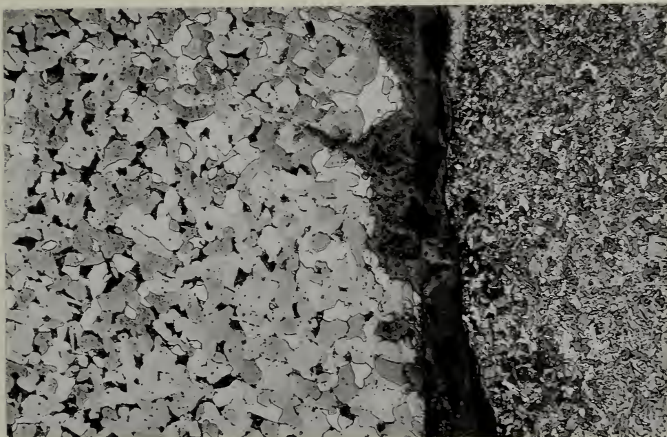
Figure 7. From left to right: hub microstructure, area of lack of welding, and heat affected zone of vane. Note decar- burization near surface of hub. 1% Nital etch. X 100
